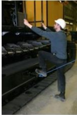
Platform Access Step and Handrail located on each side of the machine
