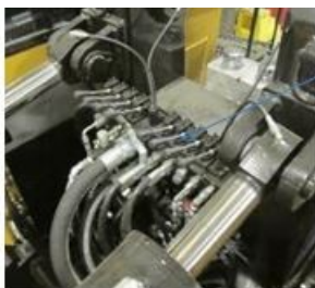
Parallel Link Valve Bank Manual Handles
