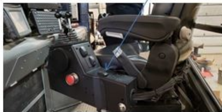
Options / Auxiliary Hydraulic Control Switches
