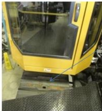
Pinch point between front of cab and platform
