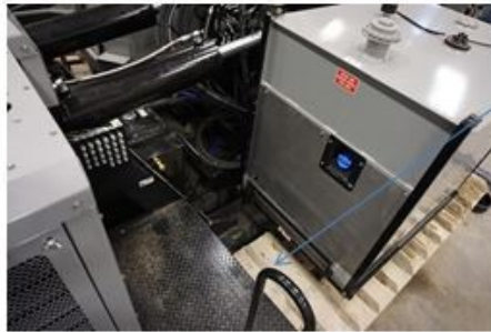
Pinch point between fuel tank mount and platform
