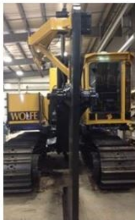
Mole swing control rotates the mole from side to side
