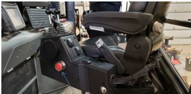
Emergency Stop Button located on the left hand side of operator's seat
