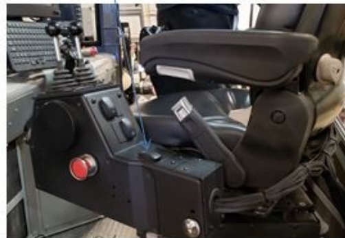
Options / Auxiliary Hydraulic Control Switches
